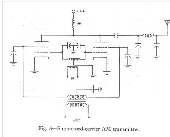
This transmitter circuit is by no means new. The information is presented here to indicate the equipment simplicity which can be realized by use of synchronous AM communications.
