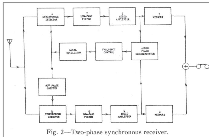
Fig. 2—Two-phase synchronous receiver.
